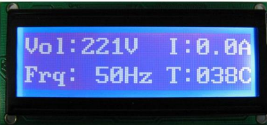
Figure 8.8c LCD screen displays information when EG8010 is connected to 12832
